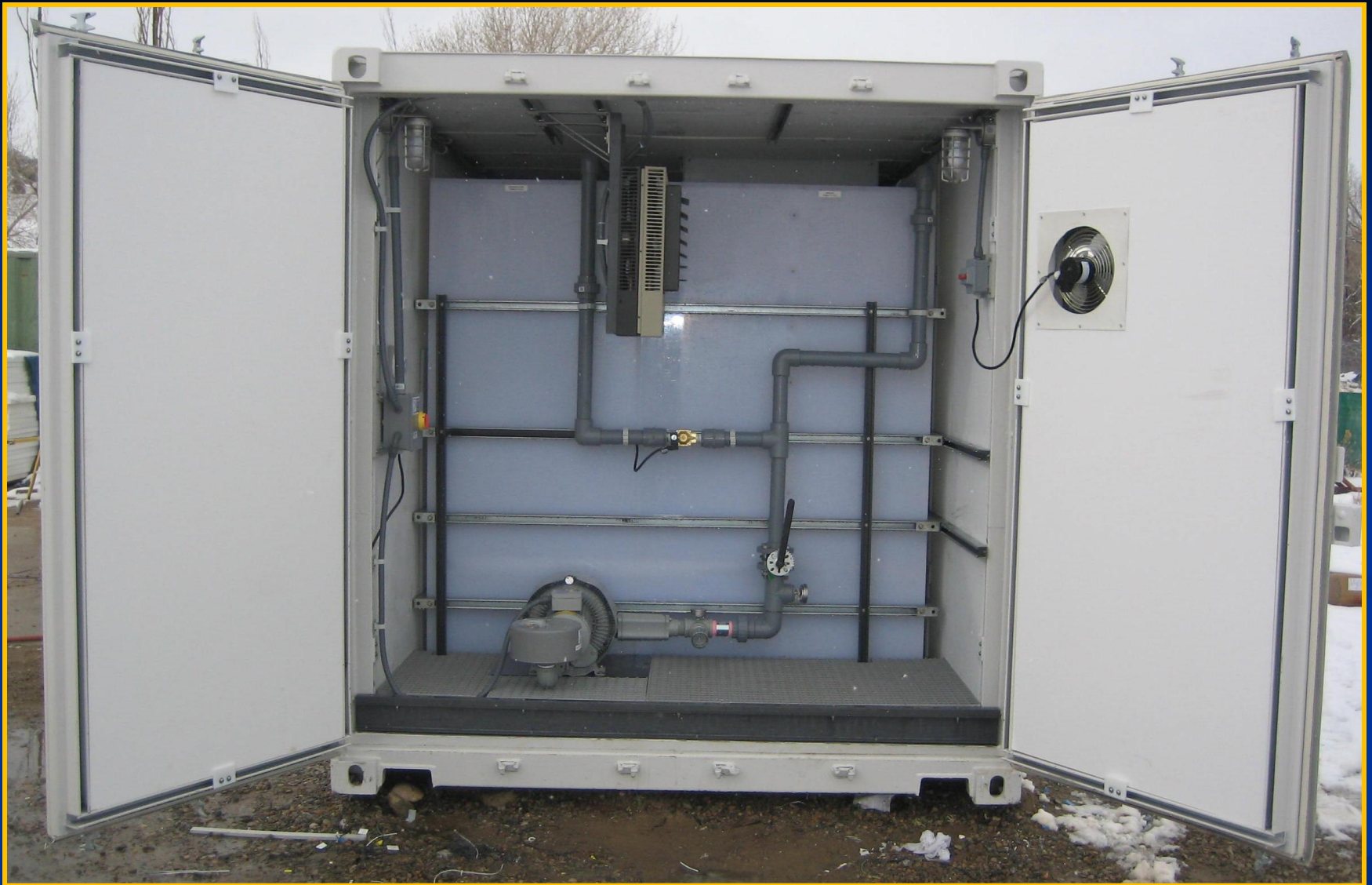
2500 GPD MBR - Entire system (including BioReactor tank) is mounted inside a 20 ft intermodal shipping container.
